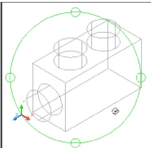
*Inside one of the small circles to the top/bottom - Rotates around the "X" axis through the center.*
