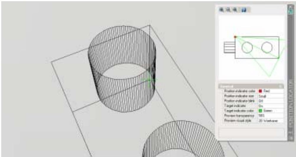
Press the Up, Down, Left, and Right keys on the keyboard to see how the camera location moves in the drawing and Position Locator dialog box.
