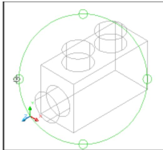
*Inside the Arcball - Allows movement in any direction*
