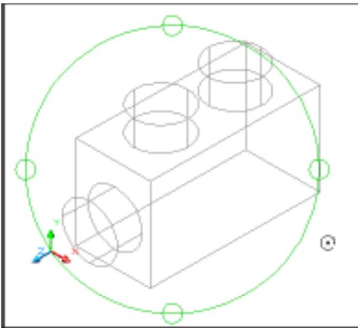
*Inside one of the small circles to the left/right - Rotates around the "Y" axis through the center.*
